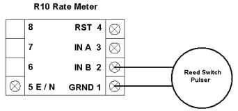
All AMCO reed switch pulsers are not polarity sensitive. Install rate meter up to 25 feet from flowmeter.
